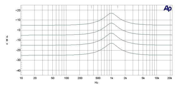
This shows a series of responses for the parametric EQ with different input levels. As expected, there is no change in the shape of the curve with different input levels. If the input is 10dB louder, the output is 10dB louder at every frequency.
